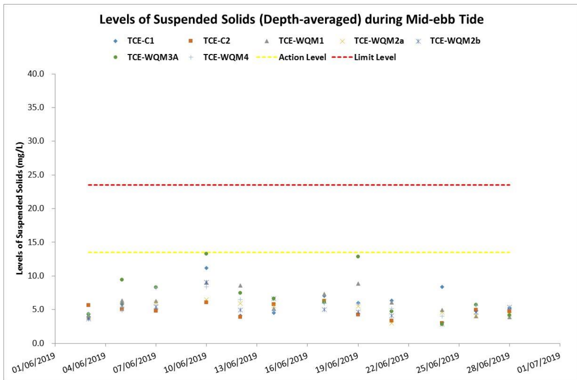
Figure 7: Levels of Suspended Solids (Depth-averaged) (mg/L) recorded at Mid-ebb Tide during the Water Quality Monitoring between 1 and 30 June 2019
